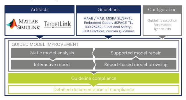
MES Model Examiner® analyzes software models for guideline compliance and guides the user through the repair and improvement process.
